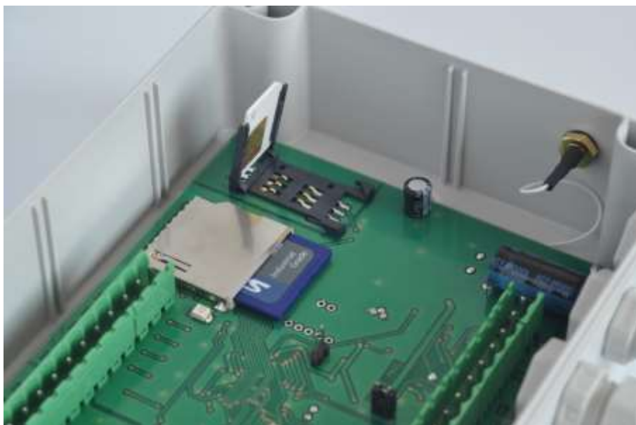
Fig 5. Observe correct orientation and insert SIM card
